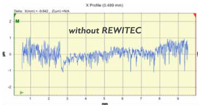
Fig. 2 and 3: Results of the surface topography in the short-term test with a white light interferometer with Agip Blasias 150
